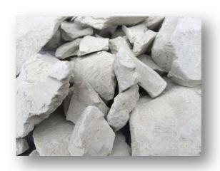
Bentonite is essentially a highly plastic clay containing not less than 85% clay mineral, montmorillonite. Excellent plasticity & lubricity, high drybonding strength, high shear & compressive strength, low permeability and low compressibility make bentonite commercially viable. There are two types of bentonites, namely, swelling-type or sodium bentonite and nonswelling-type or calcium bentonite. Sodium bentonite is usually referred
