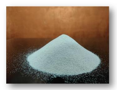
Silica sand, also known as quartz sand, white sand, or industrial sand, is made up of two main elements: silica and oxygen. Specifically, silica sand is made up of silicon dioxide (SiO2). In order to be considered a silica sand the material must contain at least 95% SiO2 and less than 0.6% iron oxide. Silica is hard and chemically inert and has a high melting point, attributable to the strength of the bonds between
