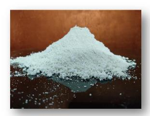
Calcined kaolin is a powdered white nonplastic material. The calcination process increases whiteness and hardness, improves electrical properties, and alters the size and shape of the kaolin particles. That makes it useful in a wide variety of products and industries. It is thus useful in refractory castables and furniture, thermal insulation bodies, low expansion bodies, permeable ceramic compositions, and investment casting. Calcined kaolins are also
