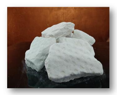
China clay is also known by the alternate name Kaolin or white clay. China clay is basically an aluminum silicate formed by chemical weathering. China clay is used as a filler material in industries such as plastics and rubber. It helps to improve the physical and physiochemical as well as electrical properties of the materials. The major application of china clay is in the ceramics and
