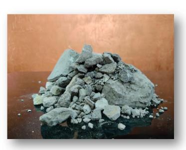
Ball clay is an extremely rare mineral found in very few places around the world. Ball clays are sedimentary in origin. Ball clays are relatively scarce deposits due to the combination of geological factors needed for their formation and preservation. Ancient rivers and streams washed kaolinite (formed from decomposed granite) from its parent rock. Ball clays usually contain three dominant minerals: from 20-80% kaolinite, 10-25% mica, and 6-
